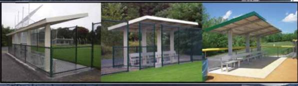
Cantilever Dugouts for baseball and softball are an affordable option that is both attractive and functional. These pre-assembled structures are manufactured with sturdy powder coated steel support beams and an angled steel or cedar shake shingle roof. The plate mounted design eliminates the need for expensive concrete footing.
